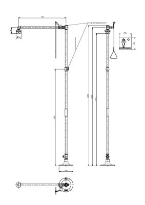
TOF emergency showers have a robust structure and are quick and easy to assemble thanks to factory pre-assembly. The valves are easy to remove, ensuring maximum ease of maintenance. The shower head produces a helical jet with a 2m diameter, fully compliant with the **DIN EN 15154 standard.**
