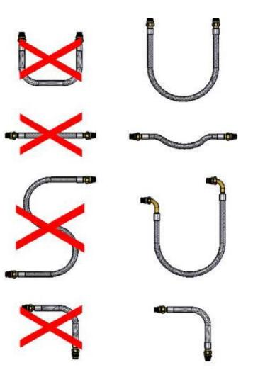
The hose/flexible pipe must have a soft bend
